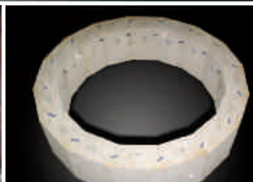
Mullite Blocks for Day Tank
